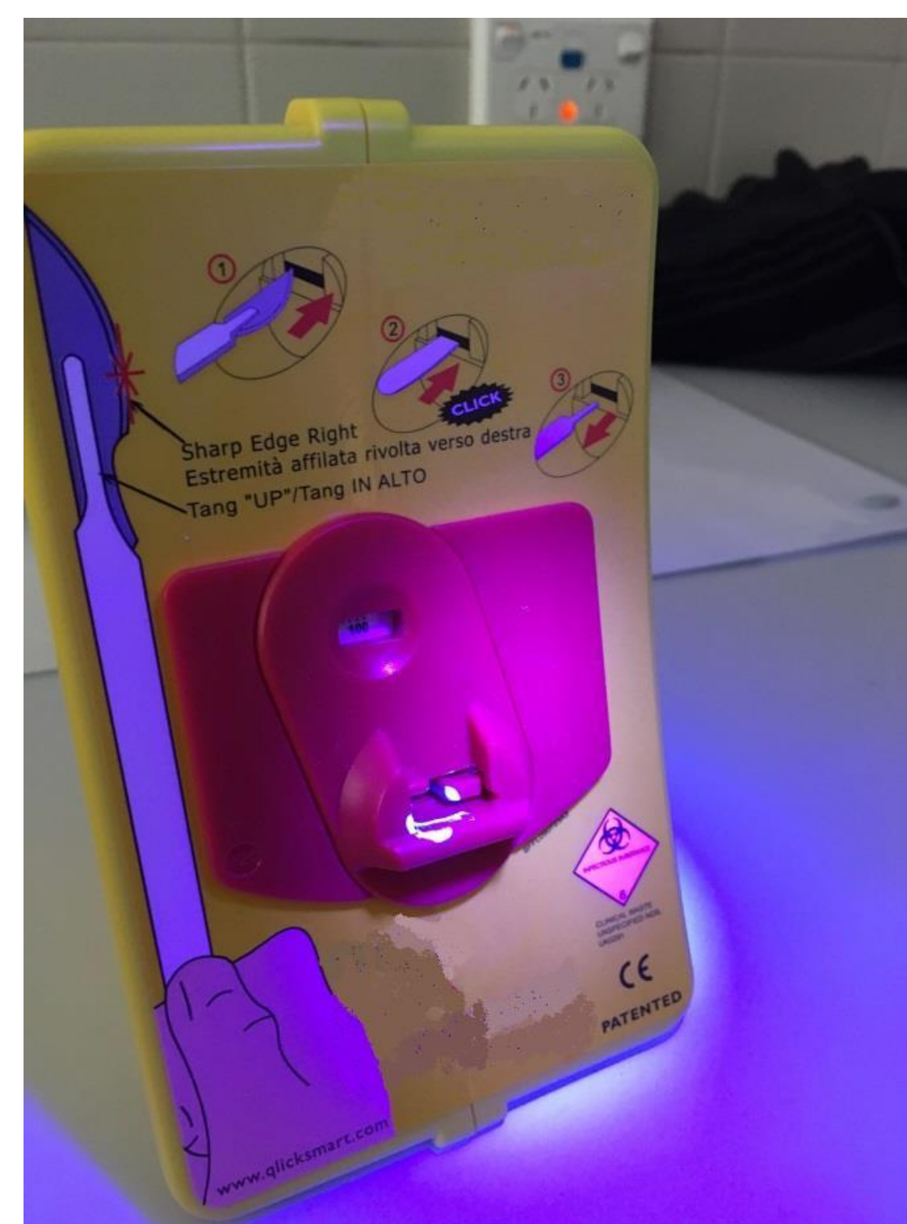
Fig.2 – Contamination on aperture of device after blade removed
