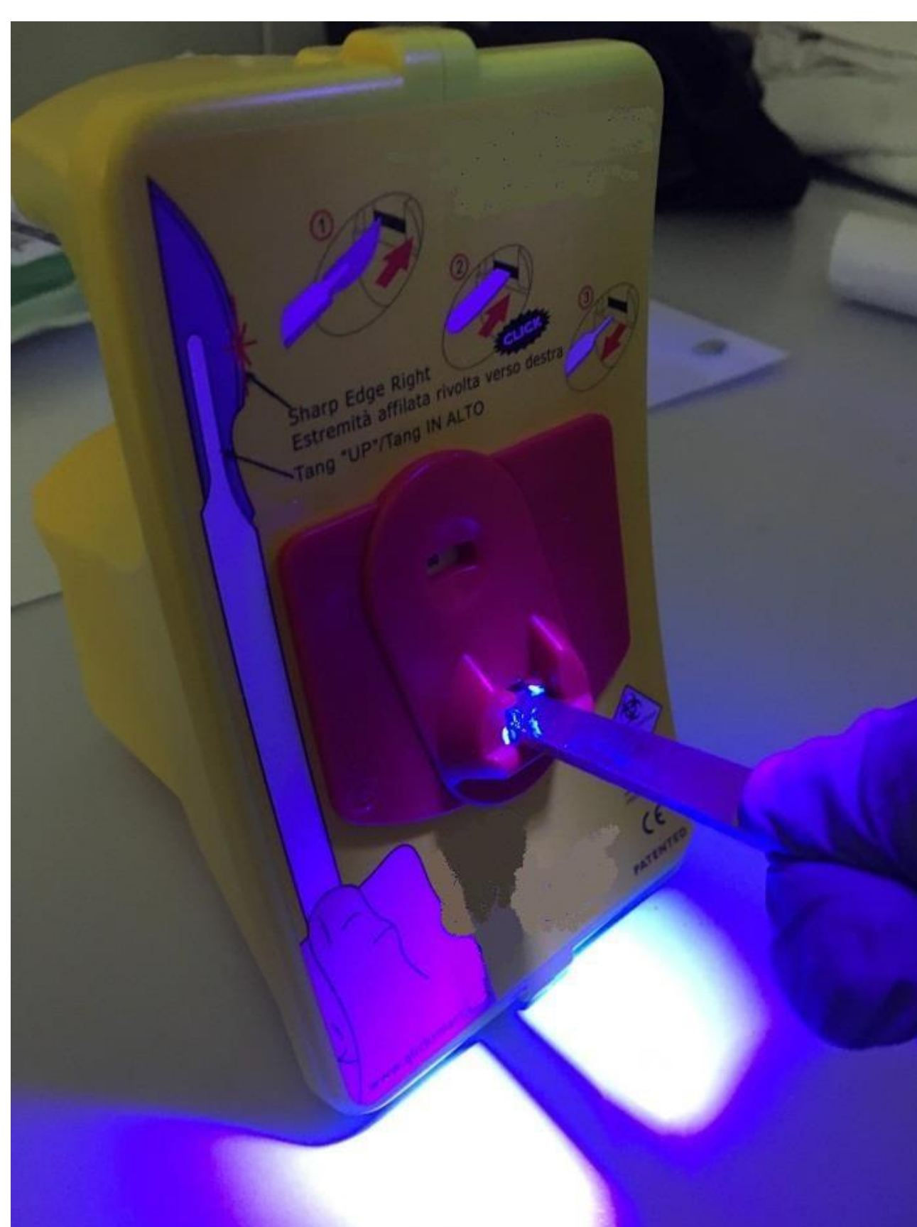
Fig.1 – Scalpel blade/handle unit with gel applied engaged with device
